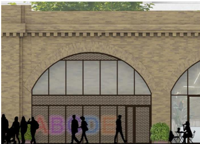
Image 50 (above): Elevation of the northern arch, showing indicatively how a scheme of lighting could be applied to the panelling.
