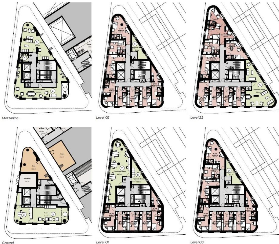
Image 37 (above): Floorplans of the six levels of the building where communal amenity facilities, depicted in light green, would be provided.
