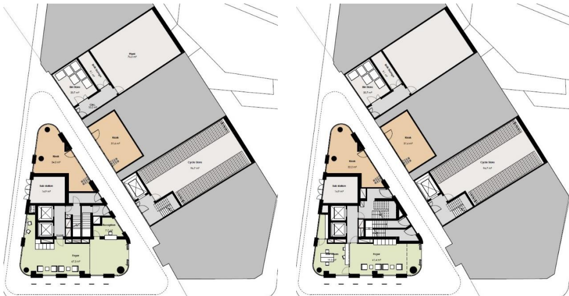
Image 20 (above): Ground floor plan at the outset of the planning application, showing one staircore within the tower.
